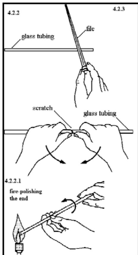
glass tubing. Placing thumbs opposite the scratch, apply force with thumbs and snap the tubing away from the body using a quick motion.
